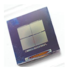
Memristor, developed by the University of Illinois and National Energy Technology Laboratory of the USA, invented by Leon Chua in 1971. Photo: Wikipedia
